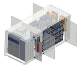
1MWh/500kW energy storage system scheme
